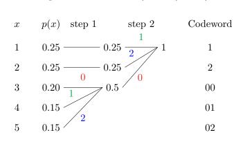
Here in each step we combine the three least probable symbols. Note that the ternary entropy of X is given by  $H_3(X) = 1.44197$ , while the expected length of the code here is 1.5 ternary digits.
