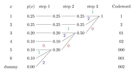
Here we added a dummy symbol so that the total number of symbols take the form 1+k(D-1). Calculate an compare the ternary entropy and the expected code length.
